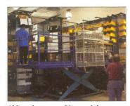
Although squeezed into a tight area, horizontal carousels have improved orderpicking accuracy while reducing labor costs.
